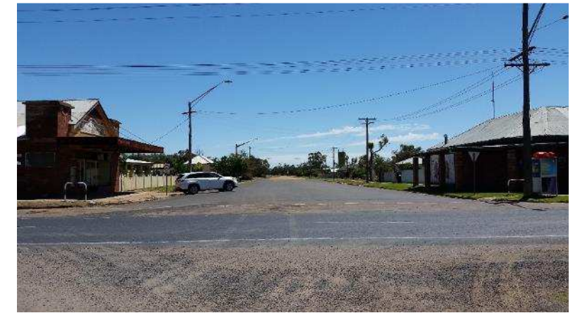
Cnr Mitchell Hwy and Clyde St (potential for wide blisters/landscape to prevent heavy vehicle entry to this street & create entrance feature)
