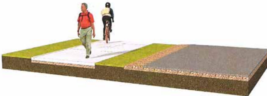
3D concept drawing – typical cross section – 2.5m wide concrete shared path
