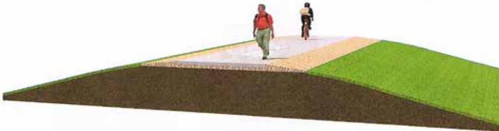
3D Concept Drawing - typical cross section - new 2.5m wide concrete shared path on existing levee bank formation
